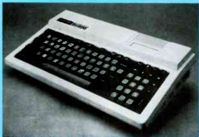
SPECTRAVIDEO'S SV-328 uses a Z80A microprocessor.
