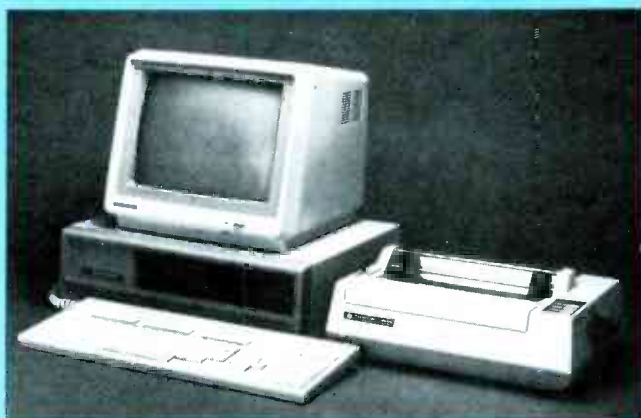
HEWLETT-PACKARD's HP200 features Motorola's MC68000 microprocessor.
