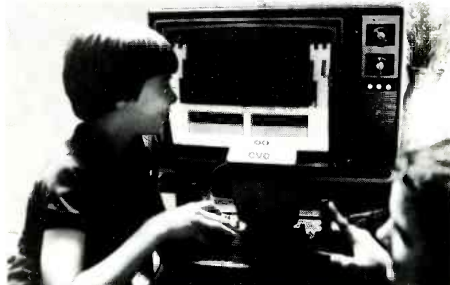
MASTER MODULE PLUGGED INTO AN ATARI VCS 2600 and connected to the telephone brings the avid player a plethora of the latest video games.
